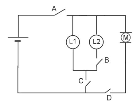
Here there is a battery on the left, a motor on the right, and two lights labelled L1 and L2 in the middle. There are also 4 switches labelled A,B, C, D.
