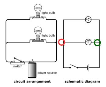
There are two paths for the electricity to go. At the **red** circle, some electricity goes to the top light and some goes to the bottom (middle) light. At the **green** circle the two parts of the current join up and go back to the battery.
