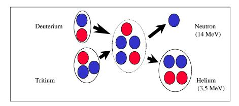
Figure I: Schematic of the fusion reaction in which deuterium and tritium form a helium atom and a neutron. Mass is lost in the reaction and energy gained.
